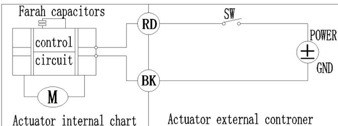
• When SW is closed , the valve open. the actuator automatically power off after in place
